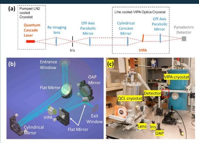
Fig. 5. (a) Simplified schematic of the main components of the testbed. (b) Detailed optical layout of the VIPA cryostat. (c) Photograph of the experimental setup in lab.
