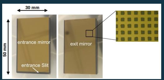
First far-IR VIPA demonstration R~16,500 (limited by VIPA length and loss in metal mesh Au layer) Current effort leading to R~100,000
