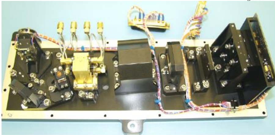
Source module Bragg-cell Imaging optics Cyl. lens CCD
