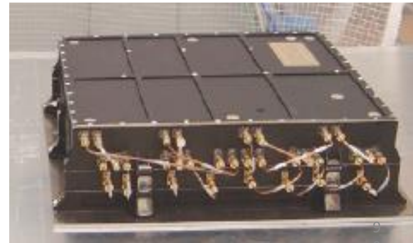
HRS (auto-correlator) with 0.125 MHz resolution and 0.25 GHz bandwidth
